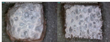
Fig. 1 Impregnated scaffolds with left 10 mg/ml and right 26 mg/ml HYALme solutions.
