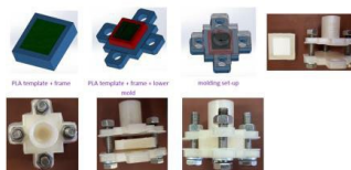
Figure 1: Indirect moulding set-up. The material is pressed into PLA mould.
