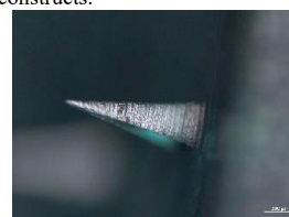
Figure 1. Optical microscopy image of a gel-MA-AEMA-coated AUP-PCL MN construct.
