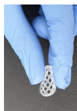
Fig.2: Printed hydrogel. Printed flexible hydrogels with web structure.
