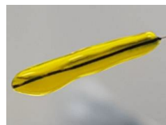
Figure 2. Picture of the PEDOT/Alginate hydrogel loaded with Fluorescein.
