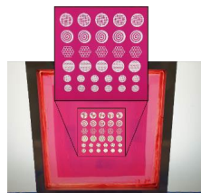
Fig.1: Screen with different geometries. Screen with defined layout of the screen-mesh. The printing paste is pressed through the bright openings and the red part is covered with photopolymer.
