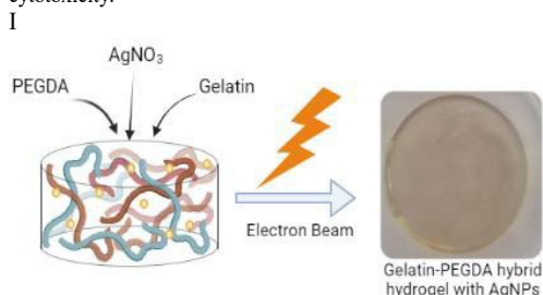
Figure 1. Schematic illustration of synthesized AgNPs/Gelatin/PEGDA hydrogels by electron beam
