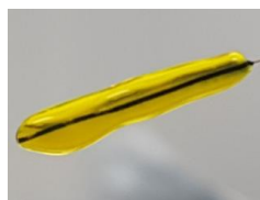
Figure 2. Picture of the PEDOT/Alginate hydrogel loaded with Fluorescein.
