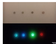
Figure 1: 3D-printed scaffolds before (top) and after (bottom) excitation under white light (Scale bar 10mm).
